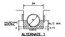
BEDDING AND HAUNCHING MATERIAL SHALL BE A-1, A-3 OR A-2-4 WHEN CLASSIFIED PER AASHTO M-145, AND COMPACTED TO A MINIMUM OF 95 PERCENT OF THE MAXIMUM DENSITY OBTAINED UNDER AASHTO T-180, METHOD D.
