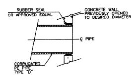
CONNECTION TO HEADWALL CATCH BASIN AND INLET DETAILS
