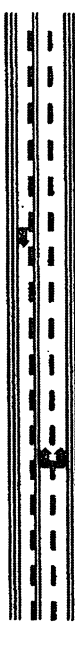
TYPICAL TWO-WAY MARKING WHERE MOTORISTS IN A SINGLE LANE ARE PERMITTED TO PASS
