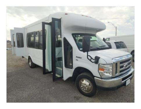
Figure 6 - Ford Econoline E-450 Cutaway Bus outfitted with wheelchair lift<sup>11</sup>
