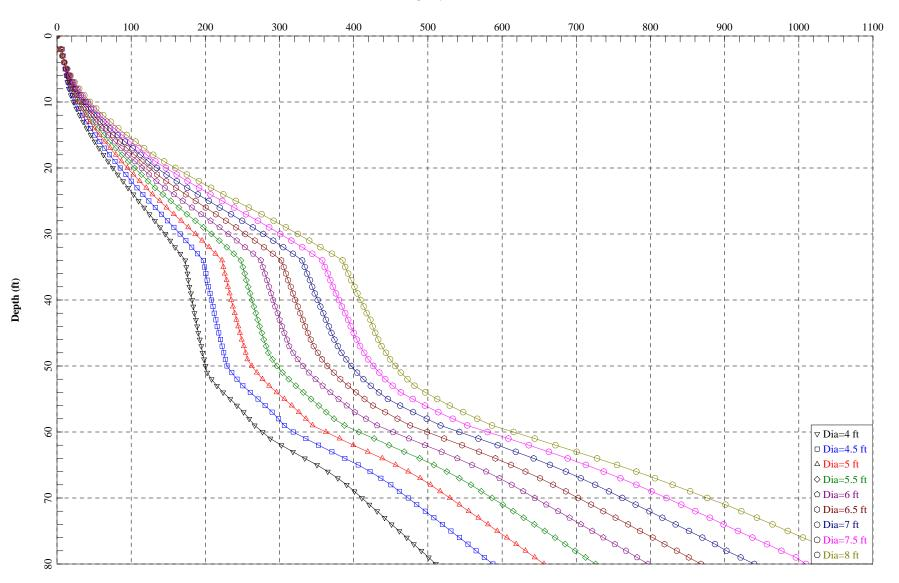
Depth vs. Allowable Compressive Axial Load - Drilled Shaft in Boring no. 1
