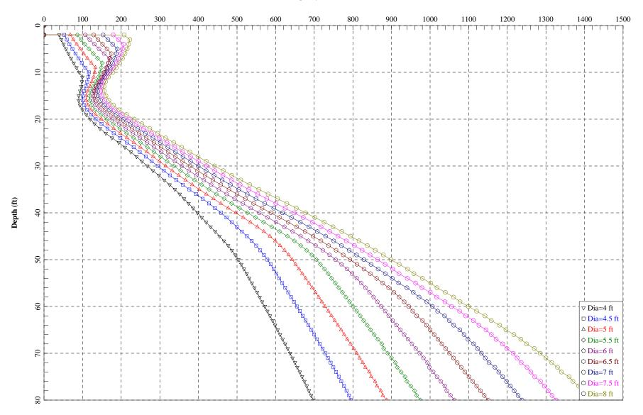
Depth vs. Allowable Compressive Axial Load - Drilled Shaft in Boring no. 6
