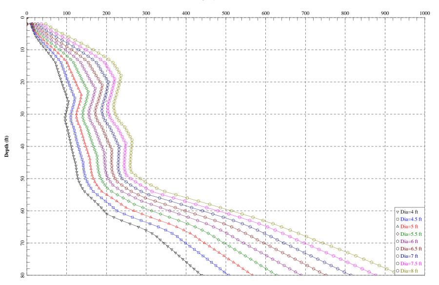
Depth vs. Allowable Compressive Axial Load - Drilled Shaft in Boring no. 5
