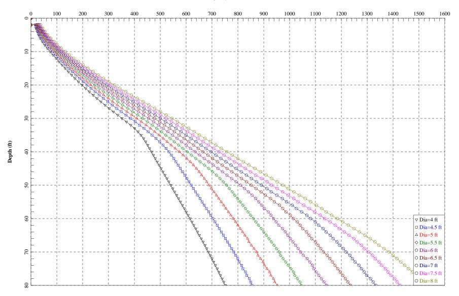
Depth vs. Allowable Compressive Axial Load - Drilled Shaft in Boring no. 2
