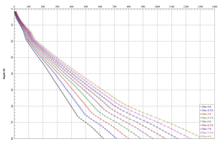
Depth vs. Allowable Compressive Axial Load - Drilled Shaft in Boring no. 3
